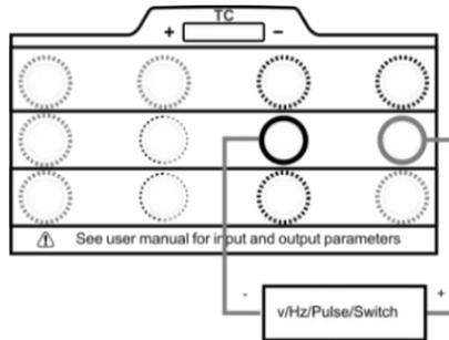
Figure 7 Voltage/Pulse/Frequency/Switch Measurement
