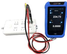
The Additel 226 non-Ex version is equipped with “true effective value” RMS measuring function, which can measure the RMS of various waveforms with no need to consider distortion or waveform parameters and other errors caused by various waveforms
