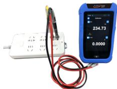
The Additel 227 non-Ex version is equipped with “true effective value” RMS measuring function, which can measure the RMS of various waveforms with no need to consider distortion or waveform parameters and other errors caused by various waveforms
