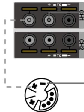
Figure 7 HART Transmitter Connection Diagram
