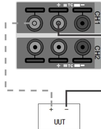
Figure 4 Connection way of Electric Current (mA) Measurement
